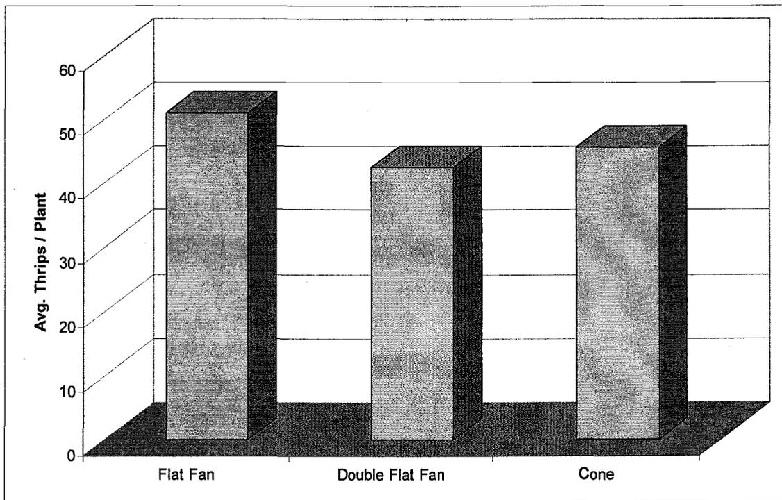
Figure 1. Comparison of nozzle design for thrips control. Malheur Experiment Station, Oregon State University, Ontario, OR, 2006.
