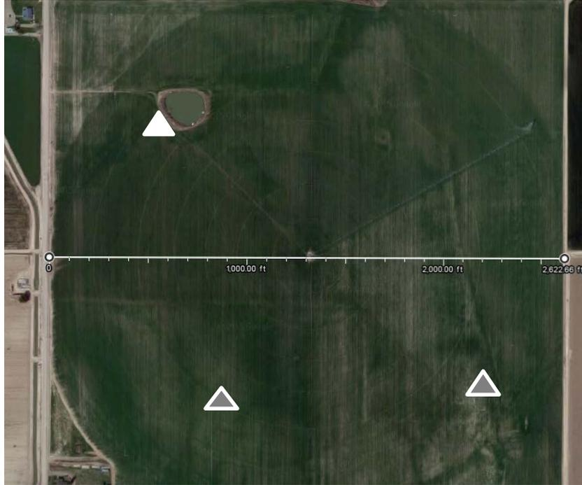
Figure 2. An example layout for a potential IRROmesh™ system. The white triangle was the location of the base station and the receiving computer. The white triangle is where a traditional site would be, the gray triangles are where the optimal sites would be. The white bar represents a distance of 2,622 ft across this field.
