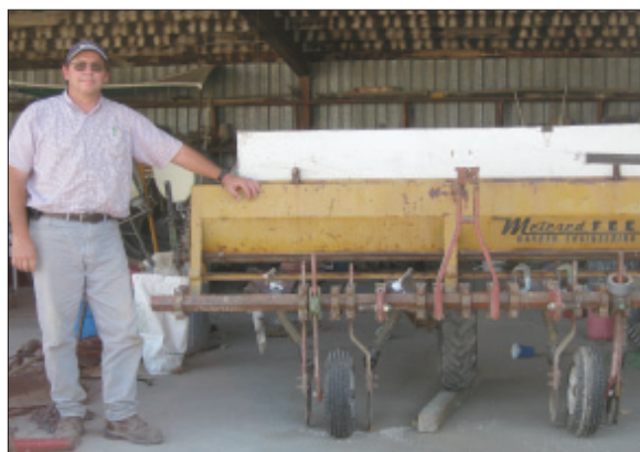
Figure 2. A sidedresser used for precise placement of fertilizer next to rows.
