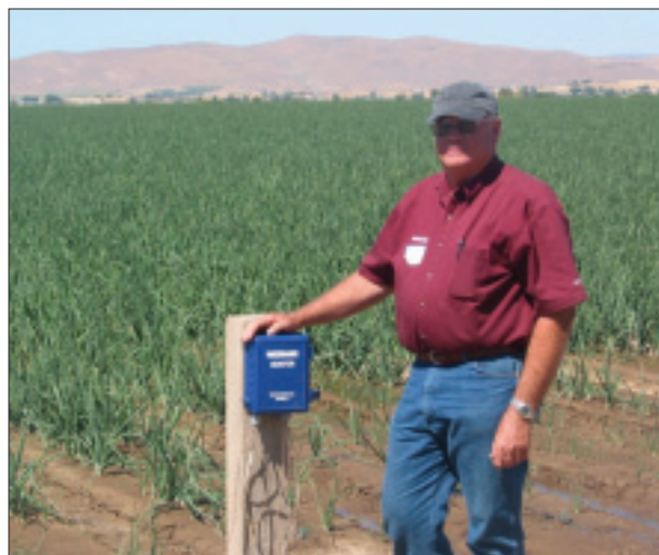
Figure 3. Irrrometer Watermark Monitor used with Watermark Soil Moisture Sensors for irrigation scheduling in an onion field.
